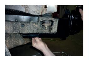
7. Using a screwdriver to hold crushed tube in position, insert long bolts with heavy duty washes through chassis bracket, chassis, crush tube and U Channel down from top.
