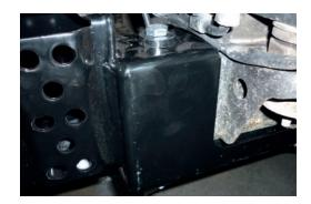
8. Install two M14 x 60mm bolts and washers through factory tie down eye into underside of left hand chassis rail.
