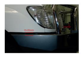
14. Once bar is aligned with vehicle and tightened drill through pinning holes between bull bar and chassis bracket and secure with hardware provided.
