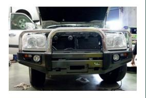
13. Align bull bar with vehicle leaving a 15-20mm gap between bull bar wing and mud guard to allow for movement between body and chassis.
