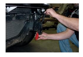
5. Place chassis bracket into position onto chassis.
